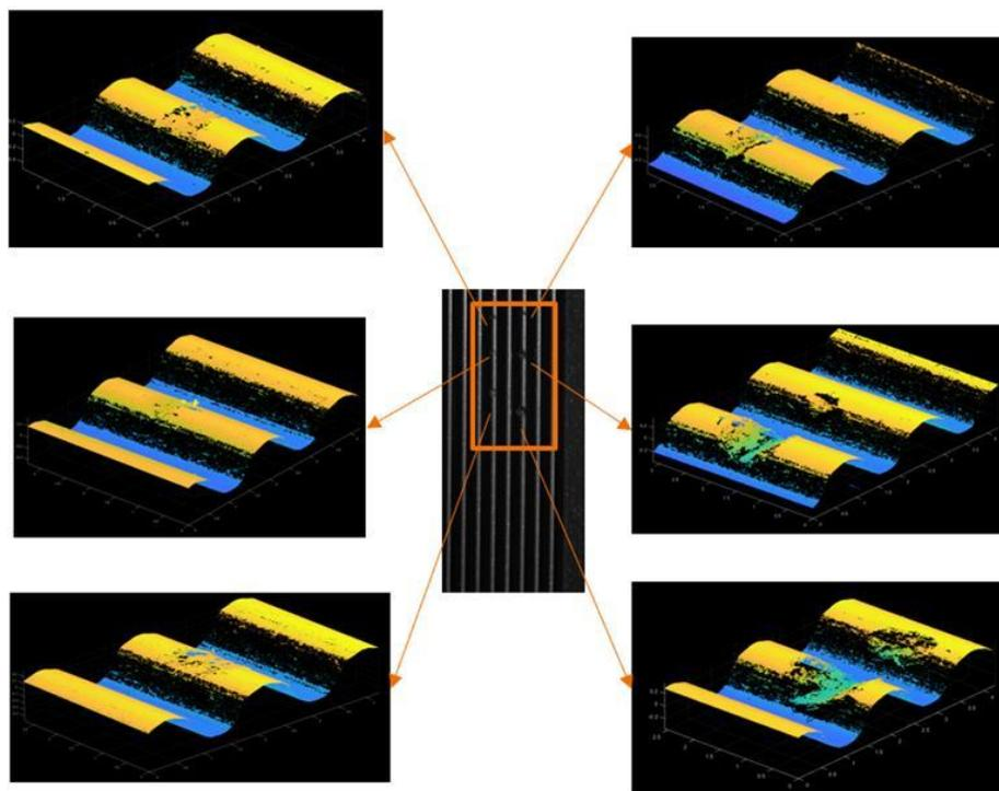
Figure 10. Illustration of appearance of defects in the dark field image and the measured 3D shape of defects.
