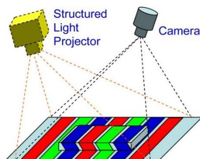
Figure 4 Structured light principle.
