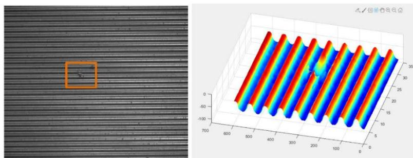
Figure 9. Illustration of a defect with diffuse lighting (left) and 3D measurement.
