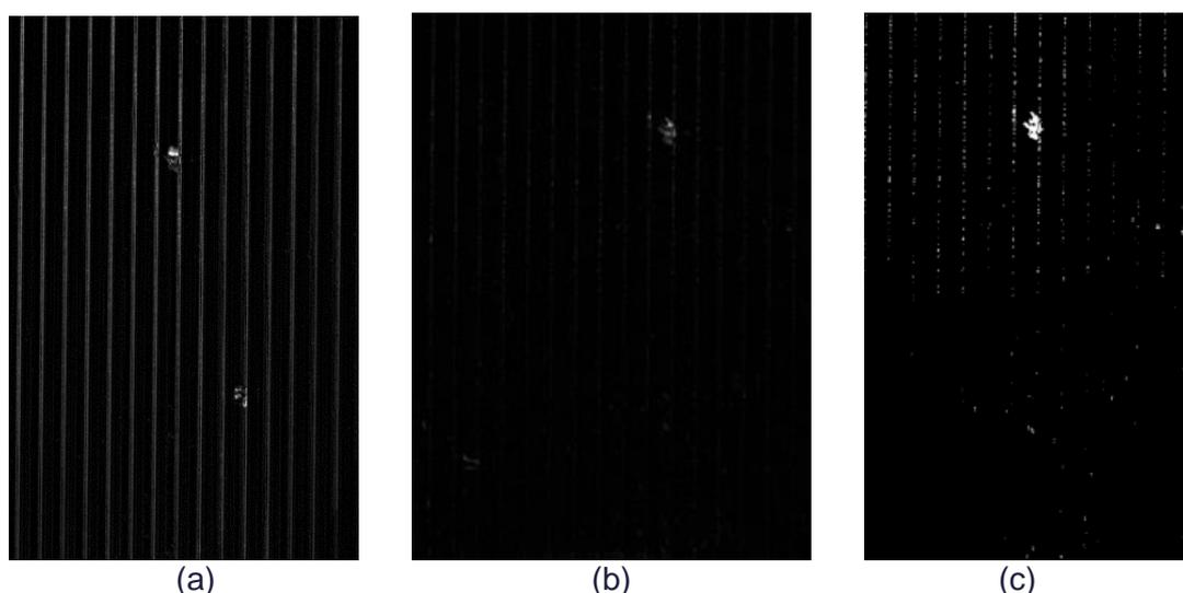
Figure 11. Image registration techniques: image difference using (a) cross correlation (b) optical flow (b). The obtained difference image can be thresholded and the result can be seen in (c).
