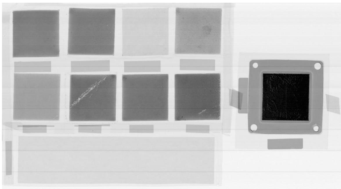
Figure 6. Illustration of Pt-loadings on square electrodes together with a full MEA
