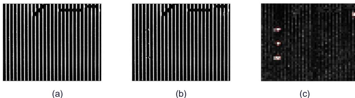
Figure 12. Illustration of (a) good sample (b) sample with defects (c) analysis based on HOG features.
