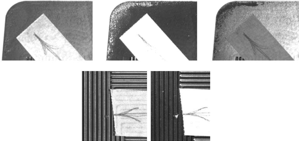
Figure 8. Illustration of the effect of different illumination patterns. Top: diffuse illumination, dark field illumination and bright field illumination. Bottom: diffuse illumination and dark field illumination
