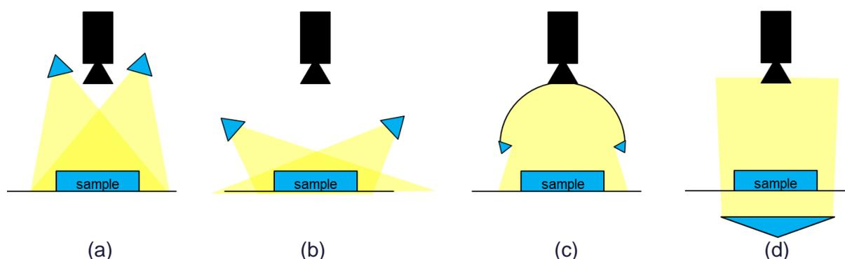
Figure 2. Illustration of typical illumination patterns. (a) Bright field illumination (b) Dark field illumination (c) Diffuse/dome illumination (d) Back illumination.
