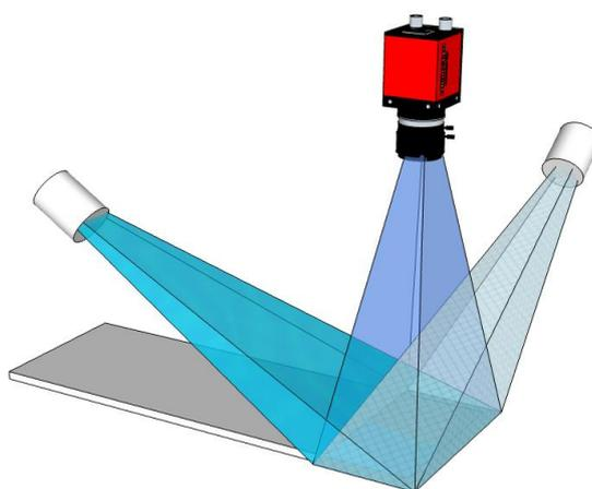
Figure 15. Concept illustration of x- and y-directed illumination and imaging of the plate.
