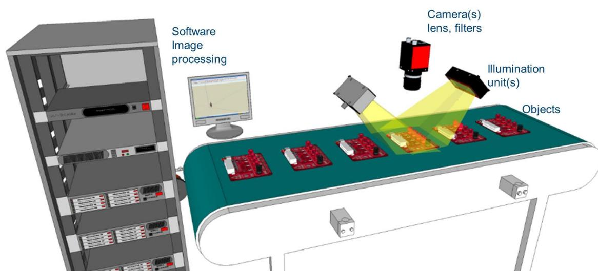
Figure 1. Illustration of a machine vision system.
