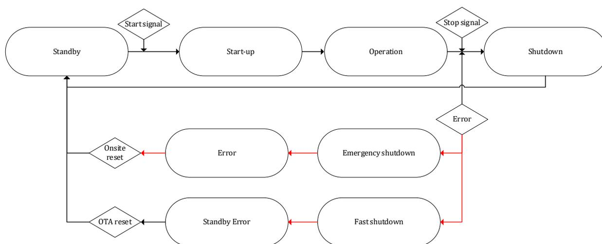
Figure 3 - Simplified state-machine illustration
